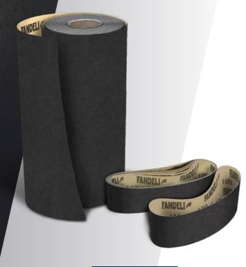
**Backing** High-resistance "F" weight paper. **Mineral** Premium Aluminum Oxide. **Grades** FEPA: P60 to P320 and P400. Coating Closed. **Ideal**
