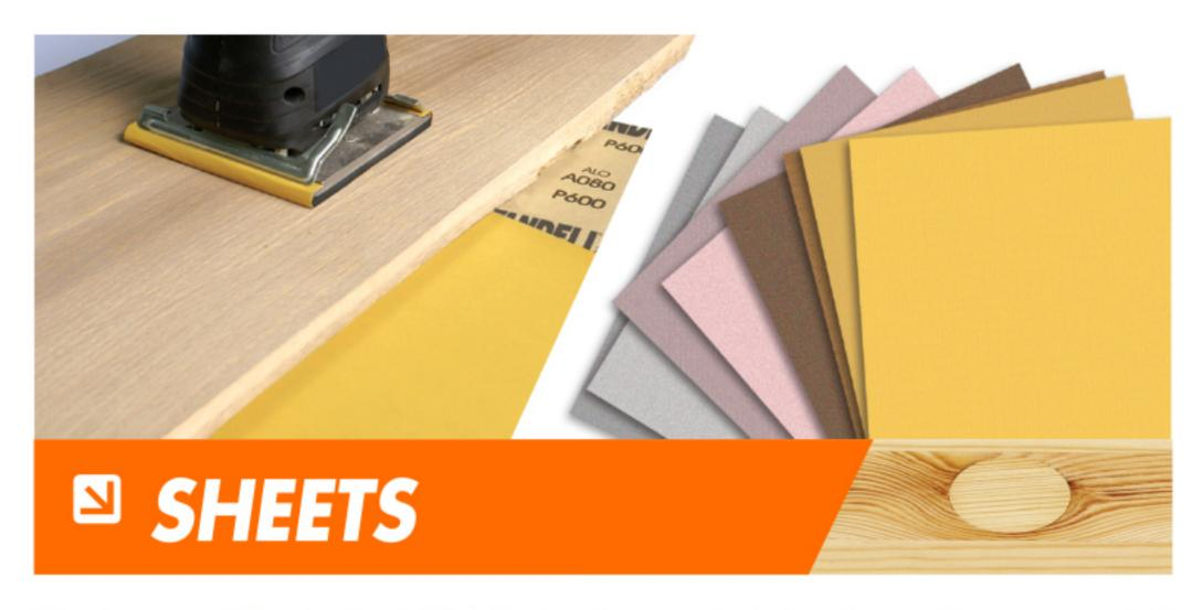
Sheets are cut in standard 9"x11" size from coated abrasives with paper or cloth backing. The choice of backing depends upon the severity of the sanding operation. Sheets are used by hand or with oscillating sanders in applications where craft is important or finishing is difficult because the parts areas are difficult to access with mechanical sanding equipment.
