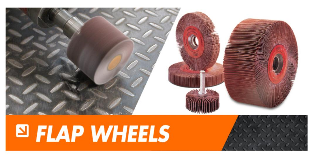
Flap wheels are made of Aluminium Oxide resin bonded coated abrasives and are ideal tools for grinding and polishing small parts, narrow curves, as well as flat surfaces. Sizes available from 1" to 6". Applications: grinding and polishing stainless Steel plates, vessels, valves, castings, welds and pipes.
